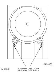
Tighten the two bolts under the drive shaft clockwise to raise the tumbler and counterclockwise to lower the tumbler. The bolts should be tightened in even increments in order to ensure that the shaft runs parallel with the base of the dryer.
